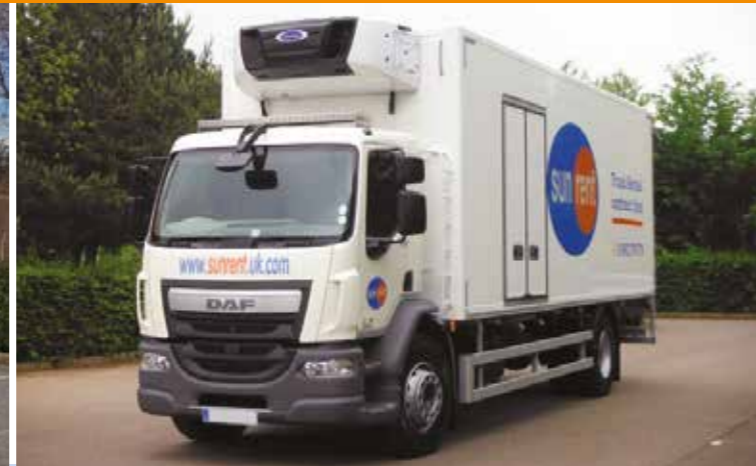
18t Box Fridge
